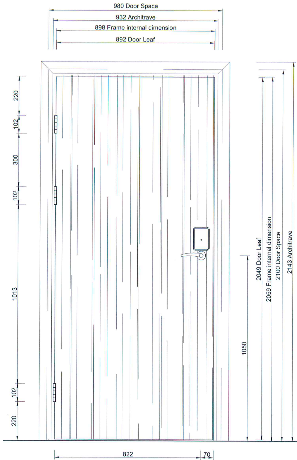
Figure 1: Exposed side view of the Door.
